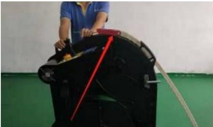
11. Remove the strap from the clamp in the chainlance and hold it straight up as shown. At the same time , move the chainlance back now by putting the joystick backward until the chain trace is approx 20-30cm lower (shorter) than the strap you are holding in your hand.
