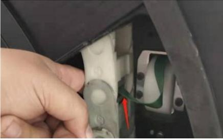
8. After releasing the chain link, make sure that the sliding window is fully closed. The safety switch of the control unit will unlock only after the sliding window is fully closed. ( When the sliding window is opened, the yellow light flashes and prompts " please close the sliding window " on the central control screen. When the sliding window is closed. the green light flashes.
